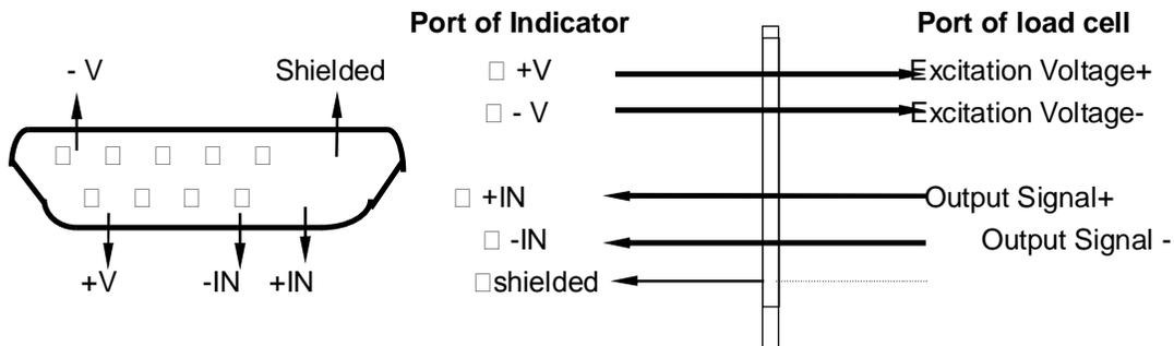
(Graph 2-3) Drawing of connecting of load cell
